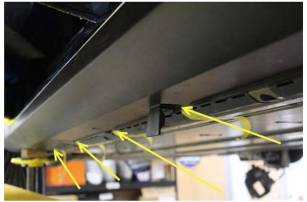
6. Remove the push-rivet clips located inside the exposed channels
