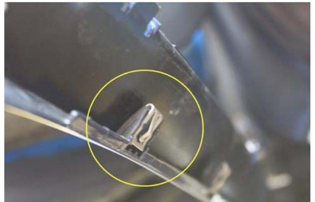
3. Next, at the front of the rocker molding, remove the plastic push-rivet clips that affix the fender liner.
