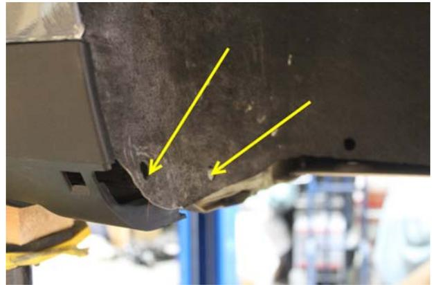
There are several push-rivet clips, as well as a screw attaching the cap to the fender liner and chassis.
