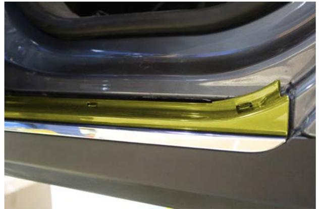
2. Next located the body-painted plastic finishing strip (highlighted in yellow). This strip is attached the OEM rocker molding using metal clips. Using a plastic panel tool, pry firmly away from the body of the car. Each of the metal clips should pop loose.
